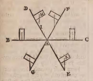
Where A, is supposed to be the place of the prop or sulciment, BC, a Leaver which stands horizontally, the power and the weight belonging unto it, being equall both in themselves, and also in their distances from the prop.
